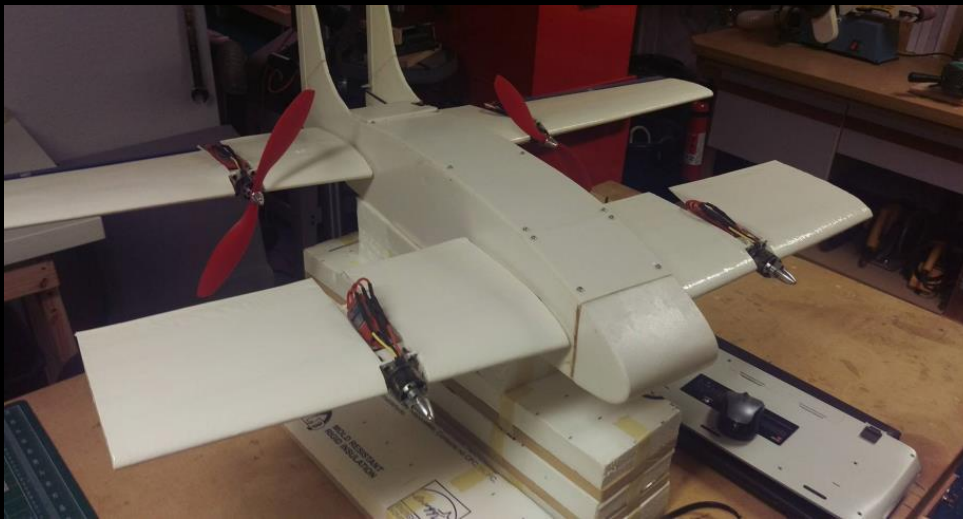
VTOL aircraft after construction, displaying independent tilt wing capabilities
