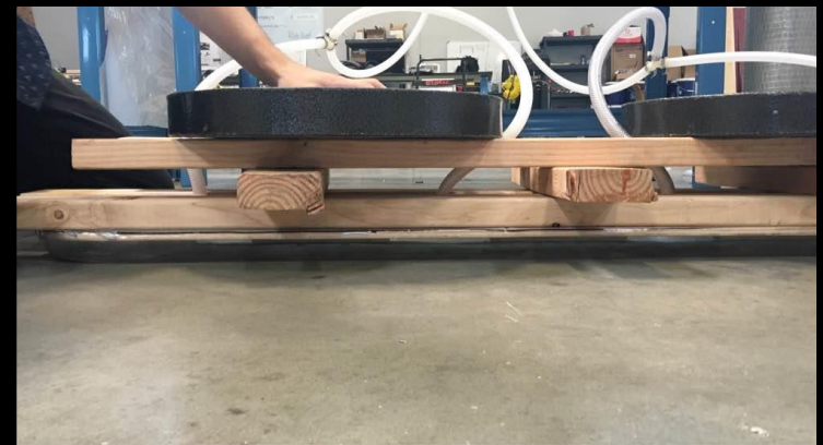
400 lbs low speed skirt test with 80 psi input
