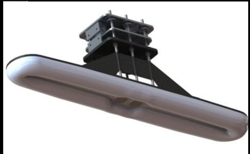
HyperXite pod design featuring air levitation
