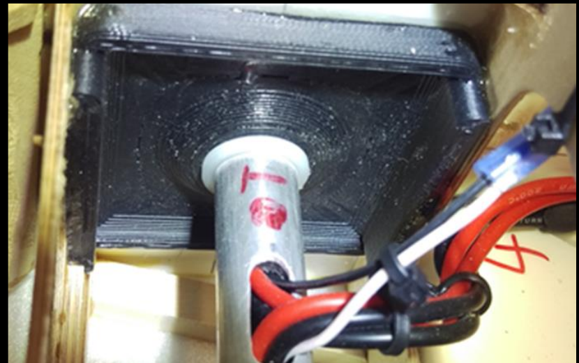
3D printed gears for wing transition mechanism and housing for nylon wing axel bearing
